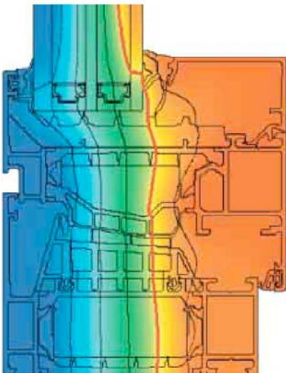
Isothermal flow in AWS 90.SI+
